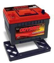
Optional height adapter may be used on 34-PC1500 models for installations where a group 24 or group 27 is required. Snap the adapter securely into place on the bottom of the 34-PC1500 battery. In some installations, the 34-PC1500 model with this adapter may be used to replace a group 24F or 27F depending on required cable length.
